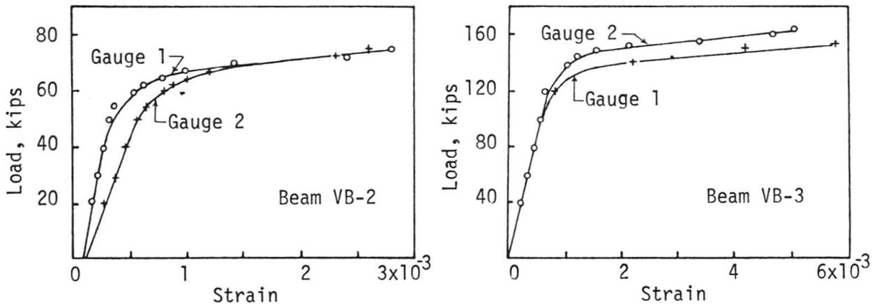
Fig. 8. Variation of compressive strain with load.
