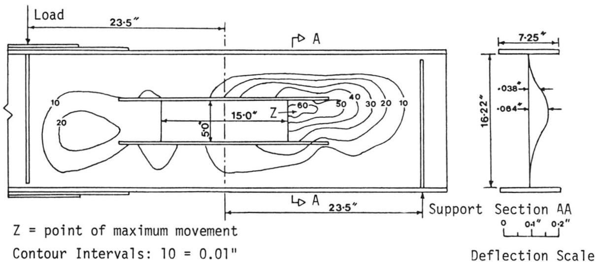
Fig. 9. Web deflection contours at 160 kips; beam VB-3.
