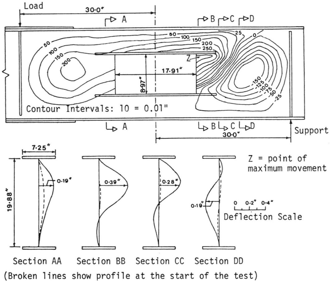
Fig. 6. Buckled web shapes and contours; beam VB-1
