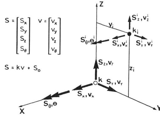
FIGURE 5 FORCES AND DISPLACEMENTS AT NODAL POINT ( $k$ ) AND SLAVE POINT ( $k_i$ )
