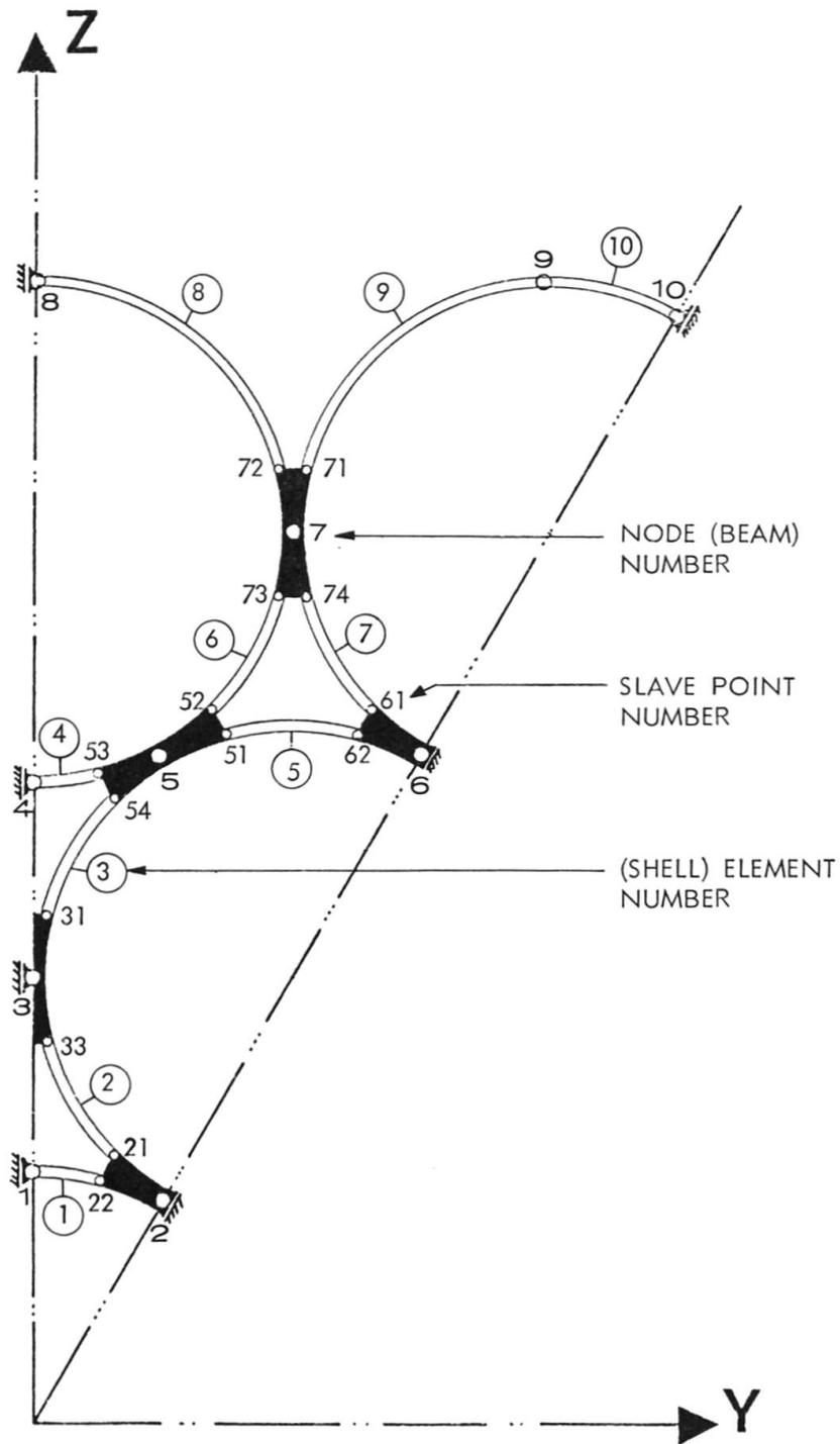
FIGURE 11 MODELLING OF THE EXAMPLE STRUCTURE IN FIG. 12
