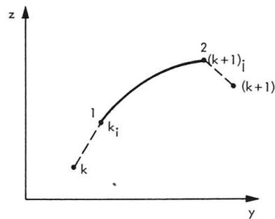
FIGURE 7 ECCENTRICALLY CONNECTED SHELL ELEMENT
