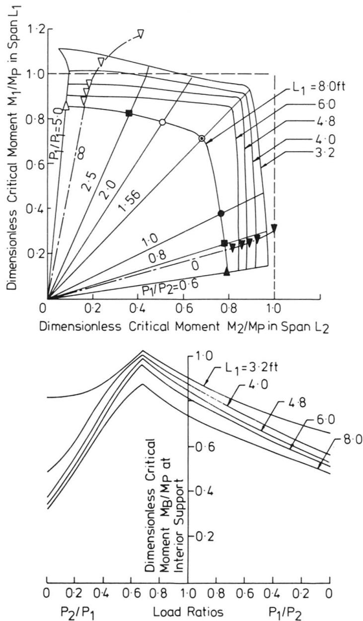
Fig. 6 Moments at Buckling in Two Span Continuous Beams
