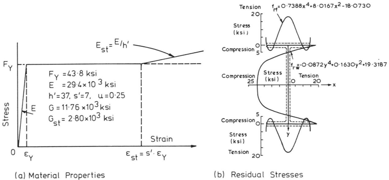
Fig. 2 Material Properties and Residual Stresses
