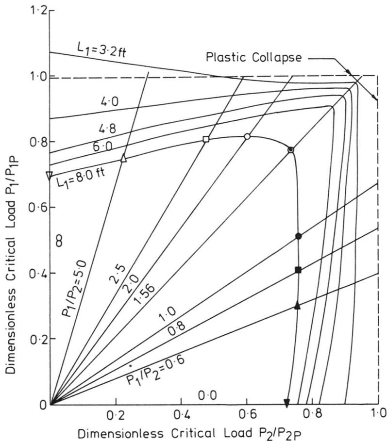
Fig. 5 Buckling Loads of Two Span Continuous Beams
