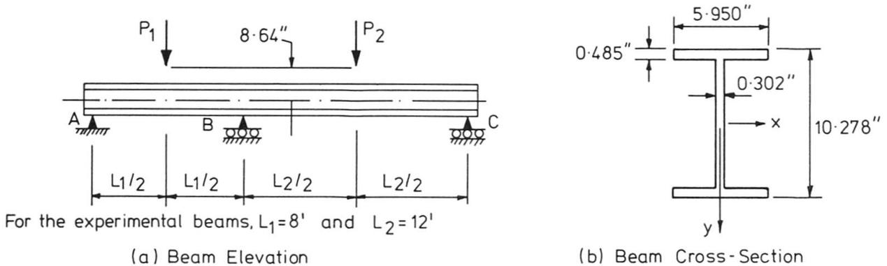
Fig. 1 Geometry of Two Span Continuous Beams
