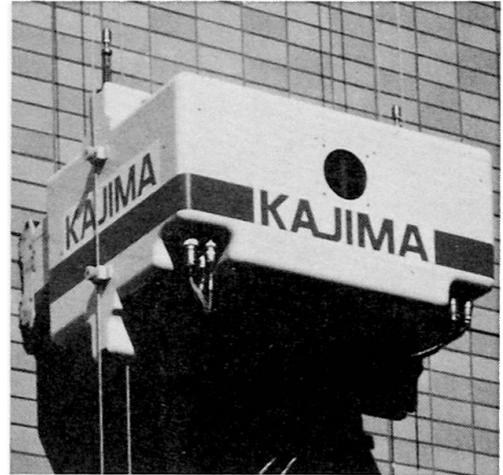
Photo 20 Tile inspection robot
