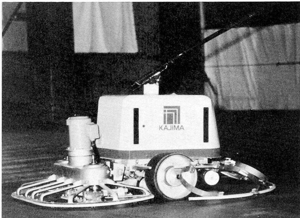
For the finishing of concrete after a slab pour, the remote-controlled motor-trowel was developed and improved to be equipped with automated sensing devices for operation. This application area is thought to be economically feasible (photos 6,7,8,9).
