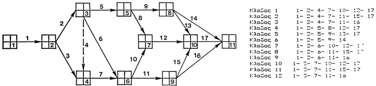
Fig.2. A network presentation with 17 activities, 11 nodes and 12 paths to be used to demonstrate the optimization algorithm.
