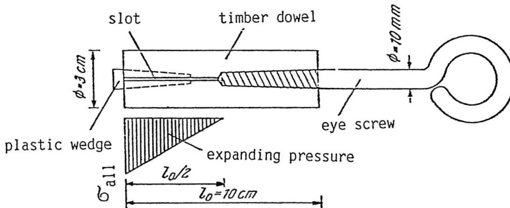
Fig.3: timber dowel and transfer of extraction force
