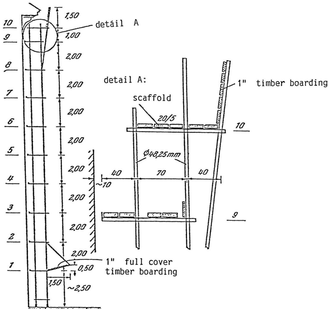
Fig.2: cross section through scaffoldings with detail
