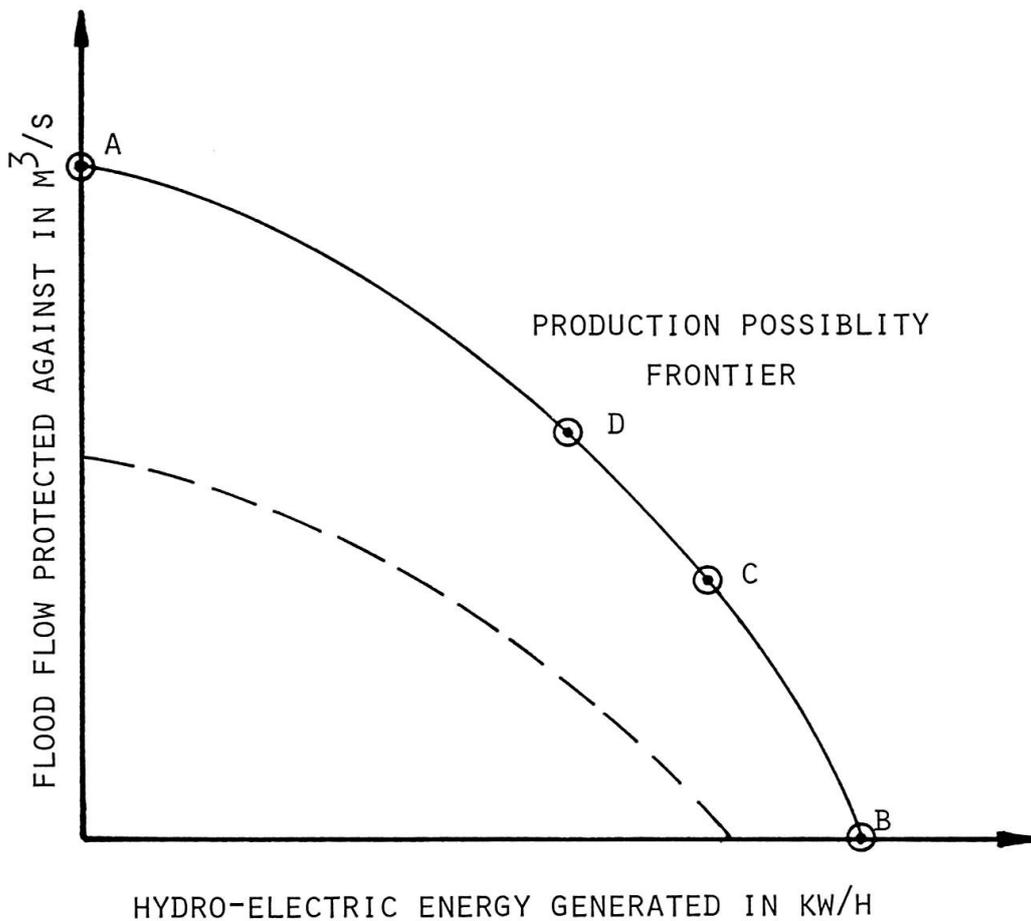
Figure 3: Flood Control and Electricity Generation
