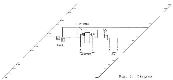
The capacity of one aggregate is 30 kg water per hour, using 44 kW for power and regeneration. The actual number of operational hours has been 440 per year, using 19,300 kWh per year per compartment.
