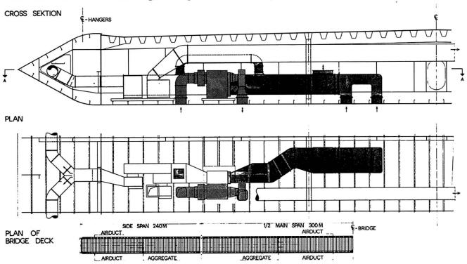
Fig. 2: Installation of the aggregate in the box girder
