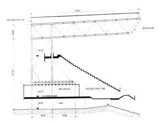
Between the beams of two adjacent cantilevers,  $24\,\mathrm{m}$  apart, lies the roof deck, made of a metallic structure with a total area of  $1100\,\mathrm{m}^2$ . The roof deck, of space frame design, weighs about  $100\,\mathrm{tons}$ .
