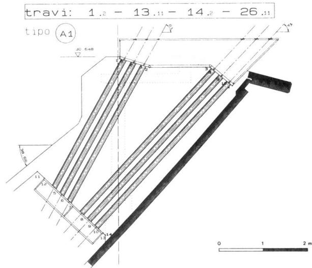
Fig. 3: Scheme of the cantilevers' connection joint
