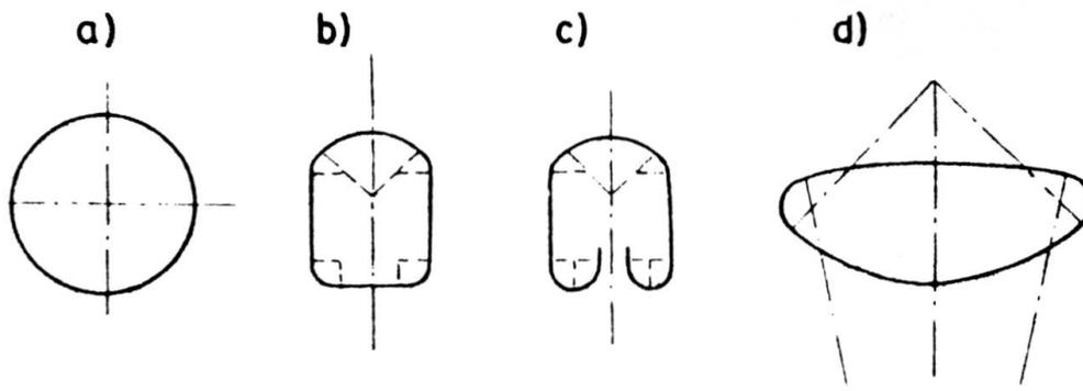
Fig. 1 Typical contour shapes of shell beams
