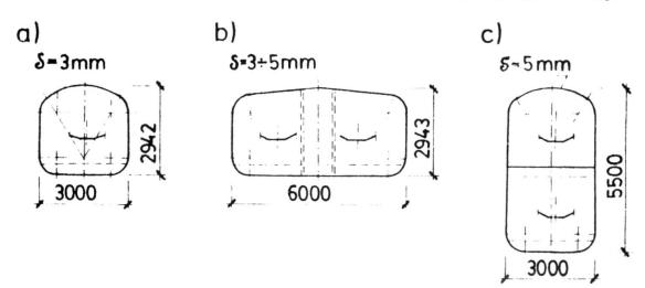
Fig. 3 Standardized contour-shapes of conveyor galleries
