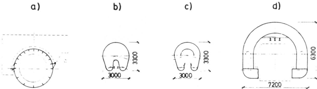
Fig. 7 Cross-sections of shell beams for travelling cranes
