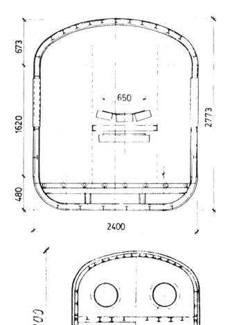
Fig. 4 Cross-section of shell beams for: a) conveyor gallery, b) pipeline bridge
