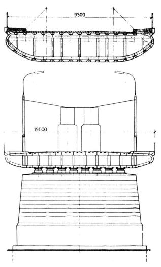
Fig. 6 Cross-section of shell beam of highway bridges:
