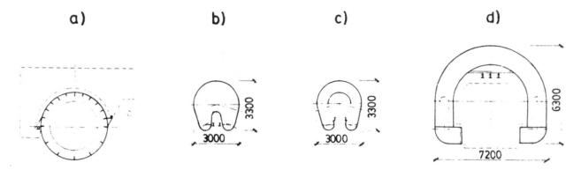
Fig. 7 Cross-sections of shell beams for travelling cranes
