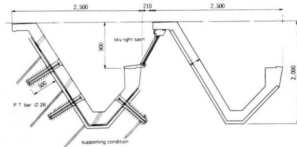
Fig. 4 Cross-section of the roof panel
