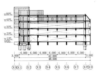
Fig. 1 Framing elevation of Y axis
