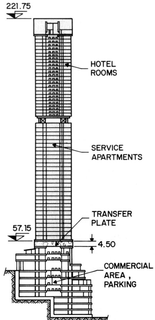
Fig. 2 Cross-section of Tower B which contains the post-tensioned transfer plate
