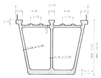
Fig. 3 Typical deck cross section
