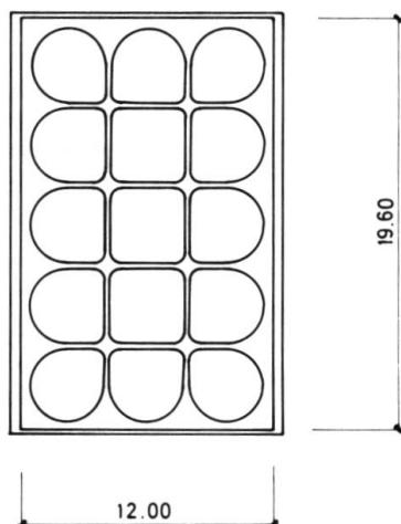
Fig. 4 Multicellular reinforced concrete caissons
