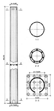
Fig. 2 Geometry of the chimney
