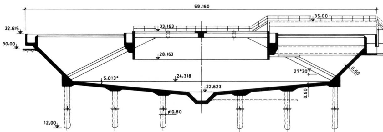
Fig. 3 Geometry of the primary clarifiers
