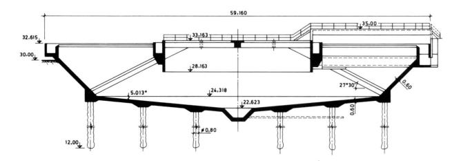
Fig. 3 Geometry of the primary clarifiers
