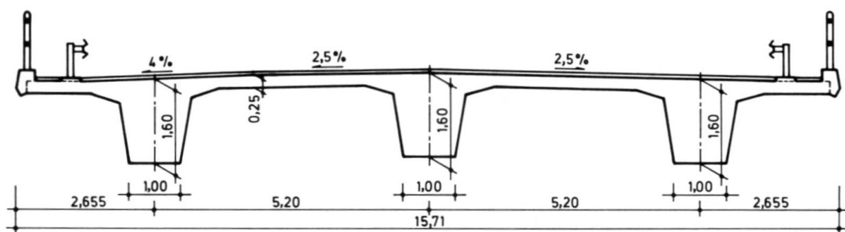
Fig. 1 Cross section type of the Bridges decks
