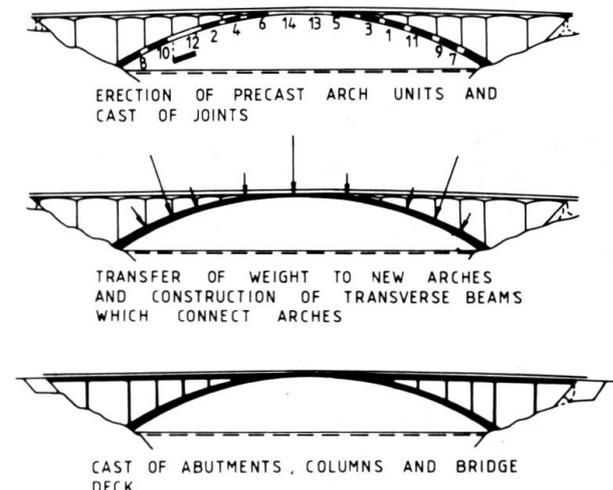
Fig. 3 Main phases of the construction process
