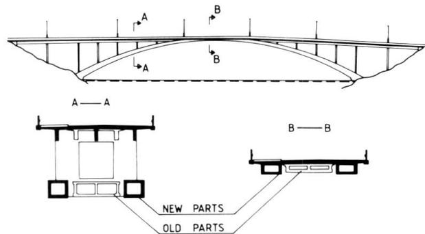
Fig. 2 Elevation and cross-sections of the bridge
