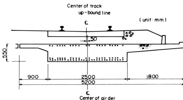
Fig. 1 Section of the girder of Wakamiya Bridge
