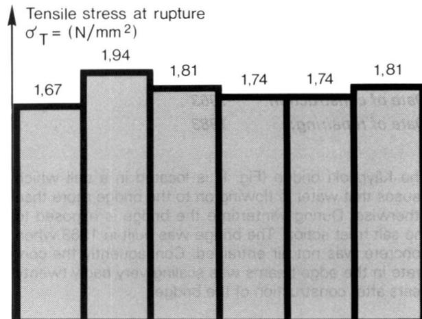
*Adhesion of the bonding measured by tests on 6 test slabs.*
