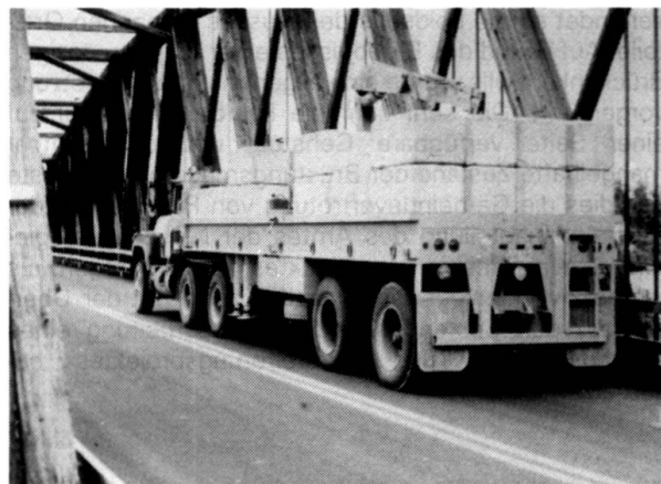
Fig. 4 Load testing the rehabilitated bridge
