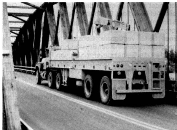
Fig. 4 Load testing the rehabilitated bridge
