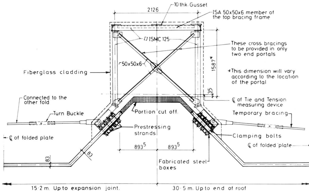
Fig. 3: Cross-Section, Canopy for extending roof at slit
