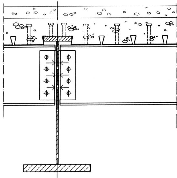
Fig. 2 The joint of primary and secondary beams
