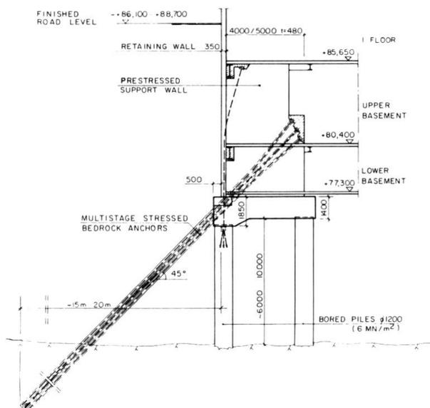
Fig. 1 The support system of the retaining wall
