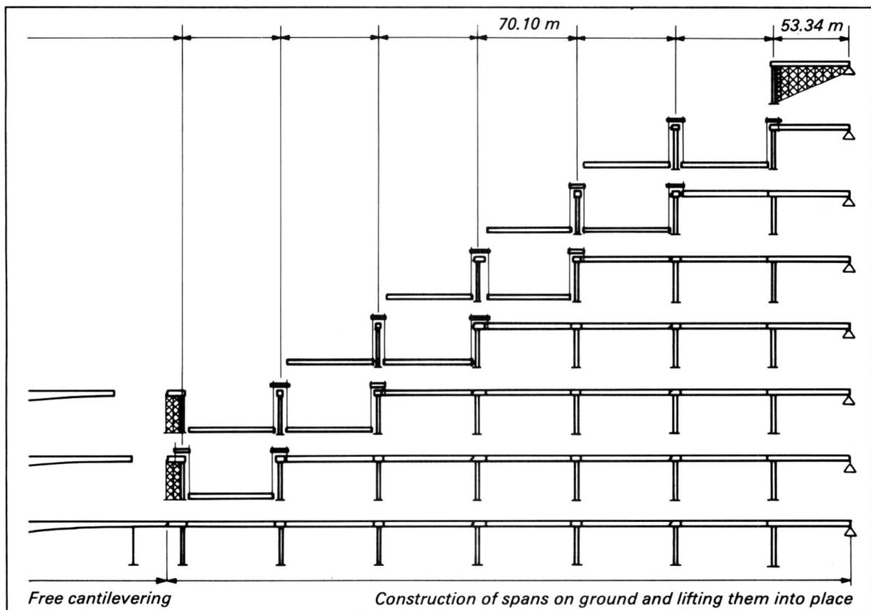
Fig. 1: Construction sequence in the approach spans
