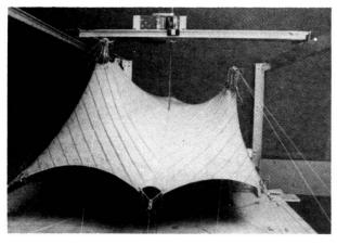
Fig. 3 Cutting pattern construction model
