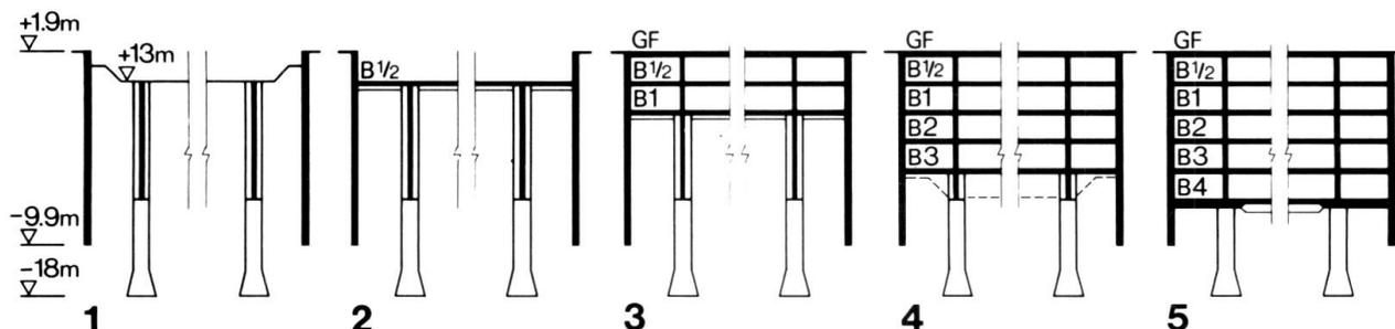
Figure 2 Top down construction of deepest basement
