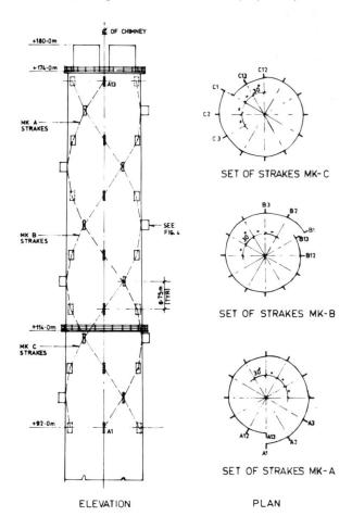
Fig. 3 Srakes arrangement
