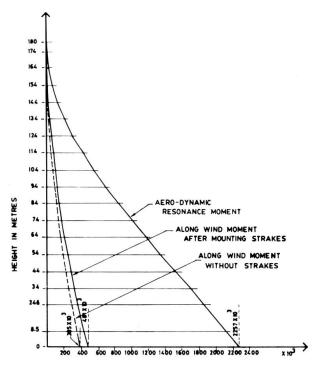
Fig. 2 Bending moment in shell in kN-M
