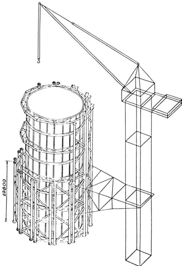
Fig. 4 The tower latticed framework and shaft erection
