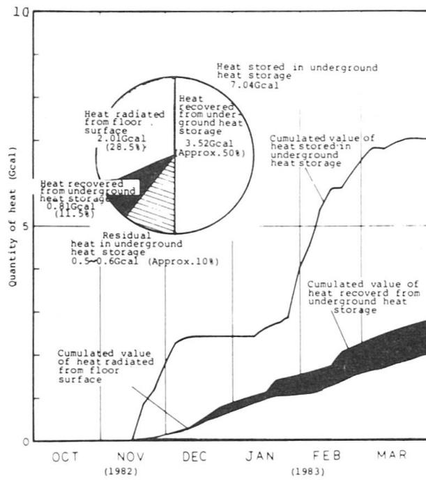
Fig. 5. Heat stored or recovered by underground coil units
