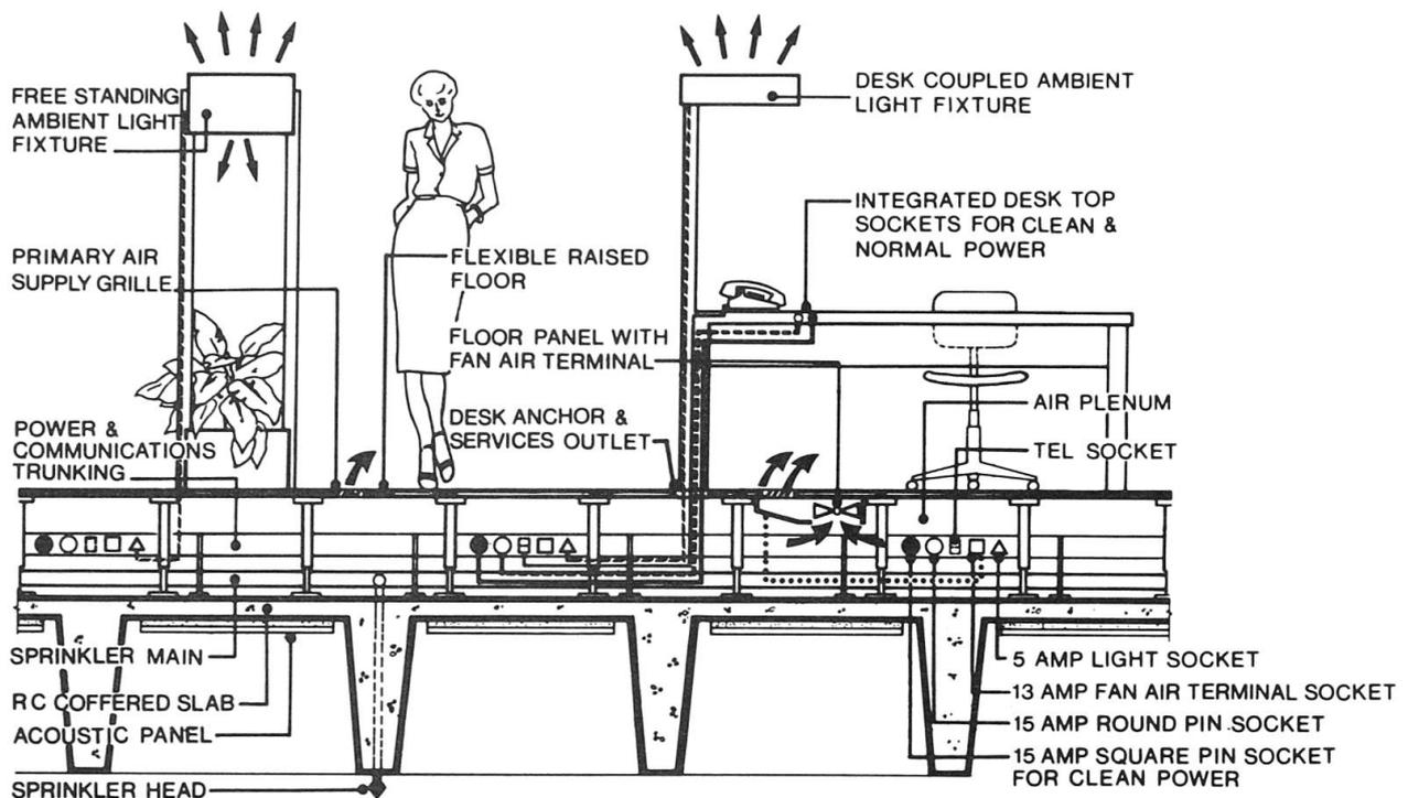
Fig. 5. Typical interface of system with workstation
