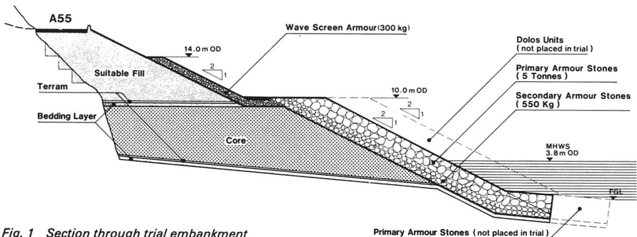
Fig. 1 Section through trial embankment
