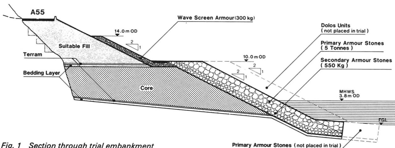
Fig. 1 Section through trial embankment
