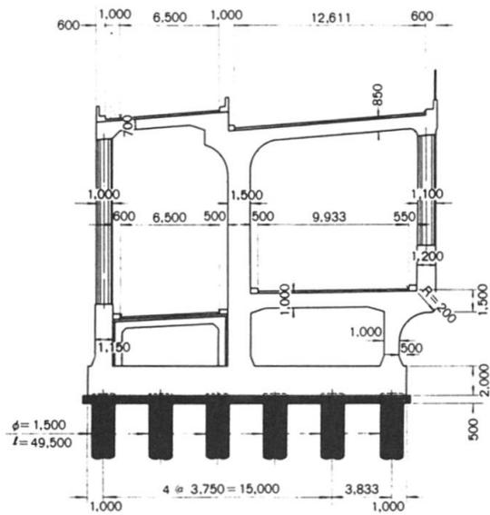
Fig. 5 Double deck section
