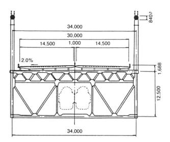
Stiffening Truss Cross-section
