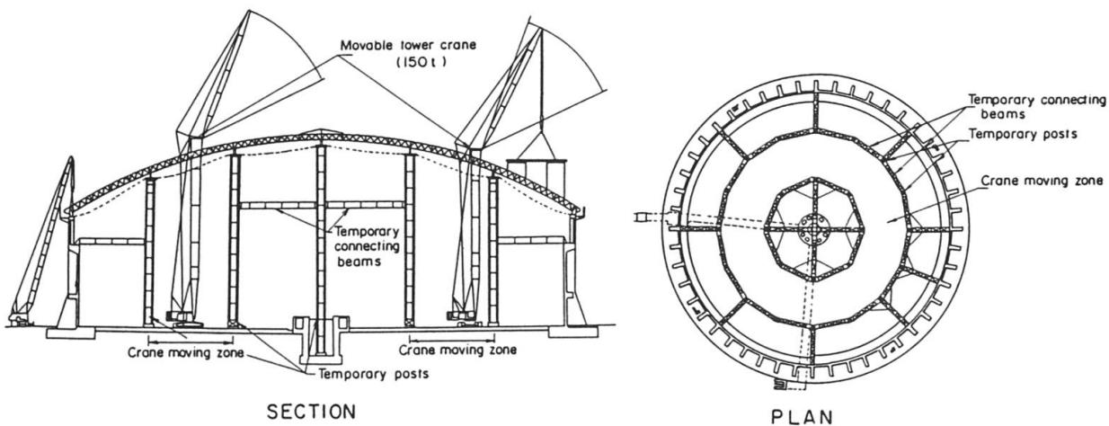
Fig. 2 Construction layout
