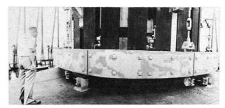
The Tower is presently extensively instrumented to allow the testing of the effectiveness of the tuned mechanical dampers and the monitoring of its structural response to wind gusting. Since completion, the tower has responsed very satisfactorily to buffetting by severe winds which occurred on several occasions registering gusts of up to 45 m/sec.
