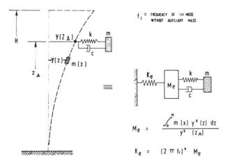
EQUIVALENT TWO - DEG. - OF FREEDOM SYSTEM FOR TOWER WITH AN AUXILIARY MASS DAMPER.
