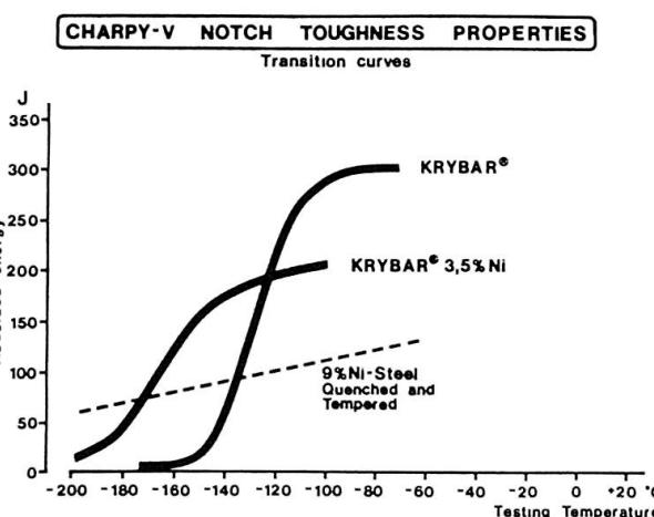
Since the original development, different material specifications have been drawn up to suit conditions peculiar to other projects i.e. ductility requirements on notched tensile bars at -165°C (-265°F).
