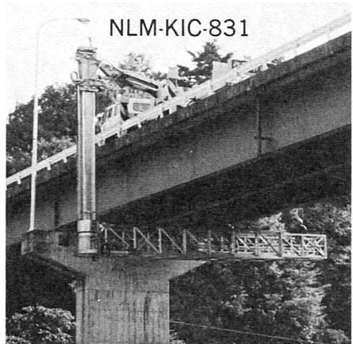
NLM-KIC-831, New Truck-mounted Telescopic Platform Type, Developed in Close Cooperation with Japan's Ministry of Construction
