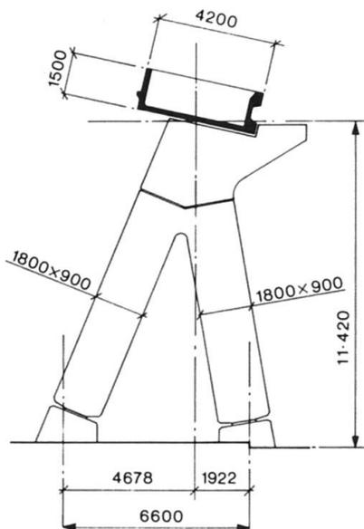
Fig. 3 Typical "A" frame elevation
