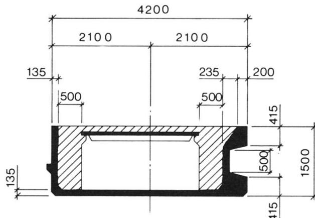
Fig. 4 Typical cross section thru ring beam
