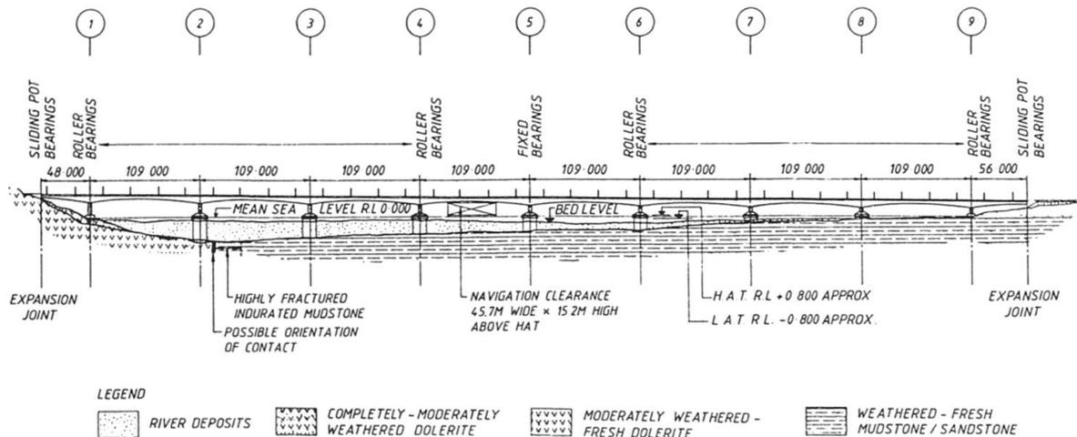
Fig. 1 Elevation of bridge
