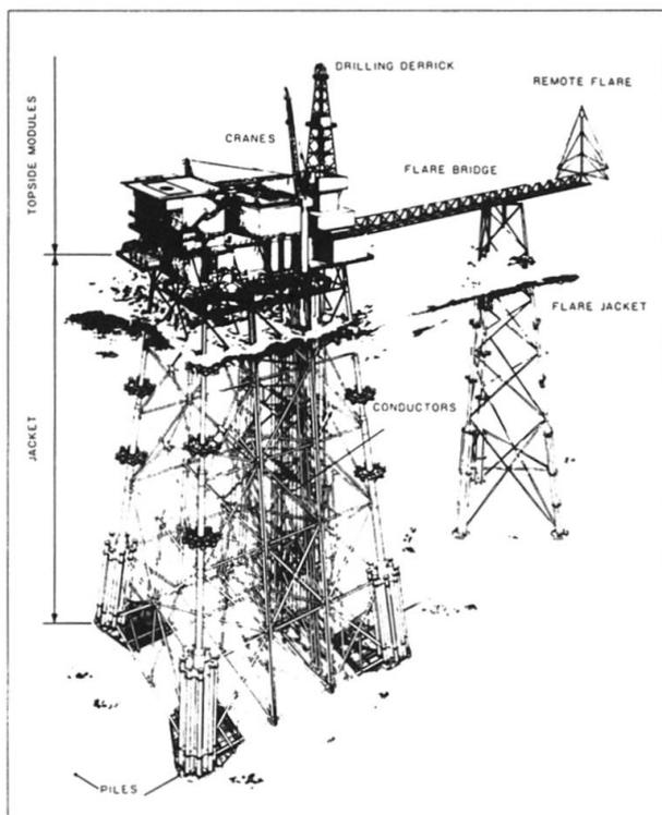
Fig. 1 Overall view of North Rankin "A" platform
