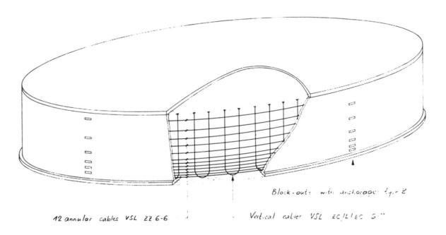
Fig. 4 Diagrammatic representation of post-tensioning
