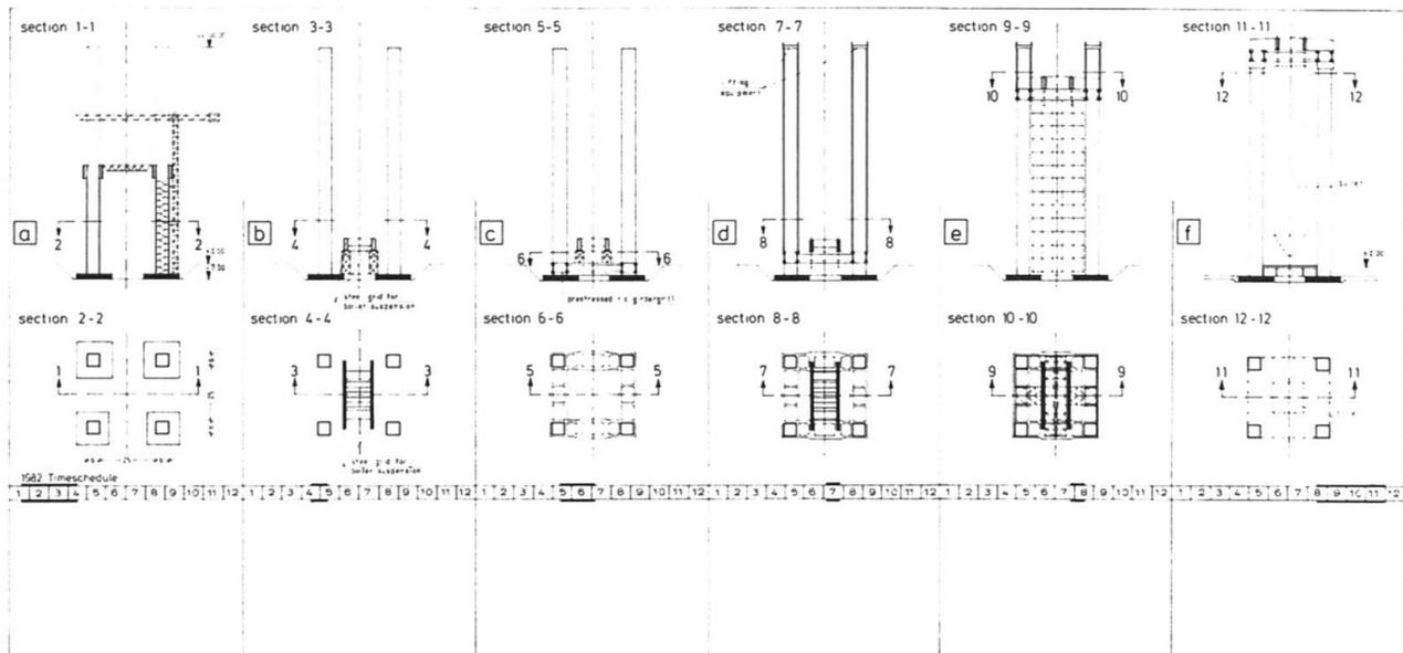
**Fig. 1** Schematic overview of the most important construction phases.
