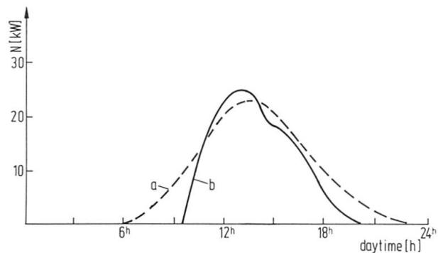
**Fig. 24:** Comparison of model calculation and measured power output. The climatic data obtained on site were used for the simulation model.
