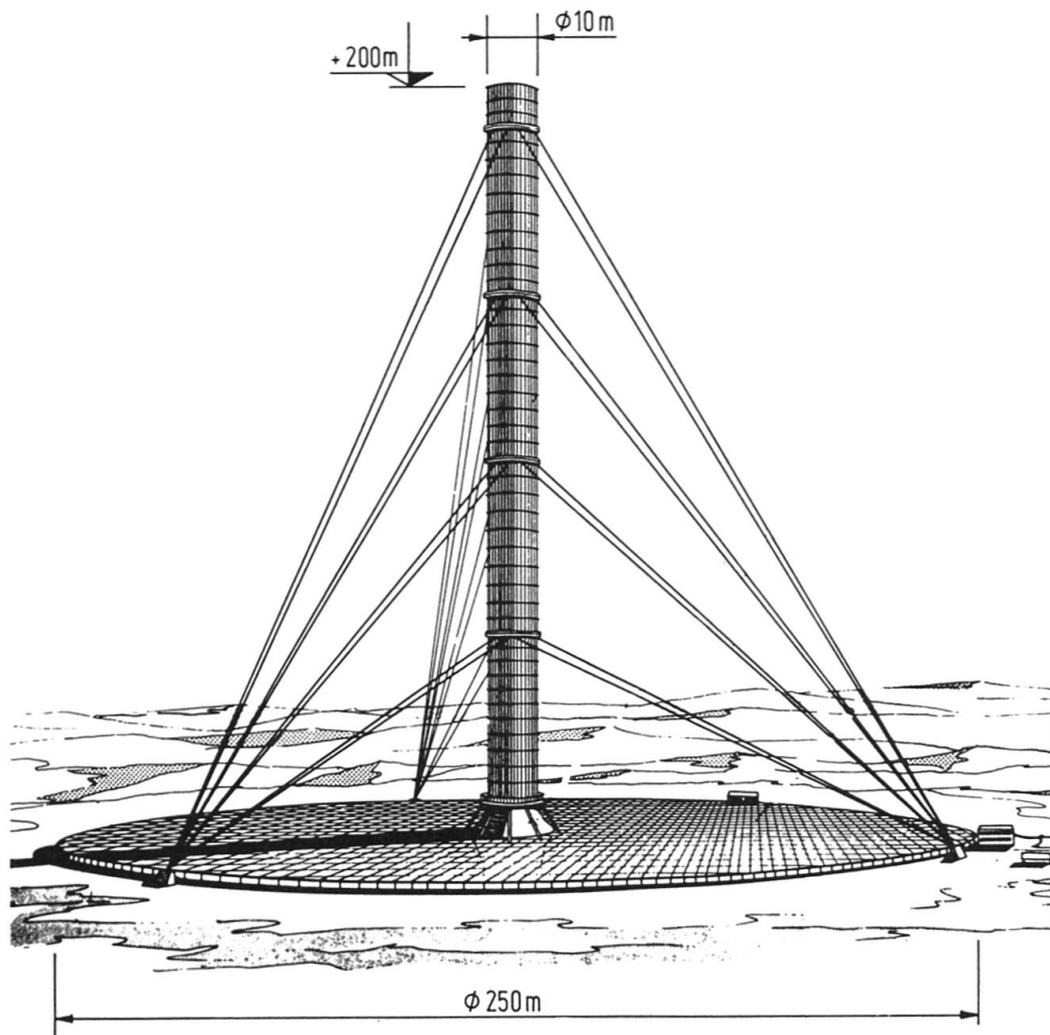
Fig. 10: Main dimensions of the pilot plant
