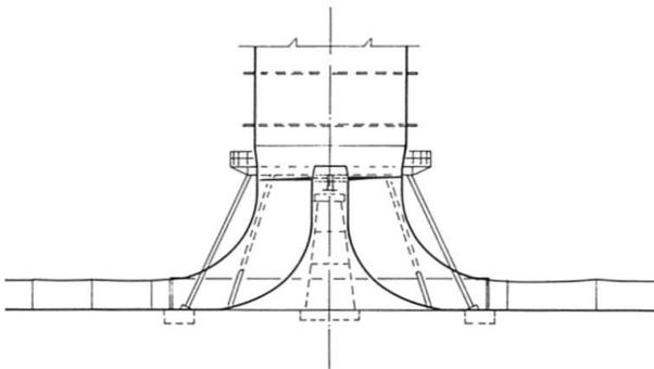
Fig. 20: Section through the base of the chimney
