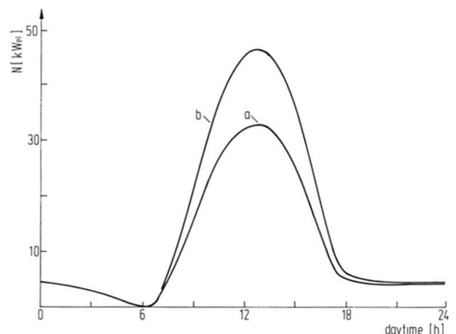
**Fig. 19:** Electricity output of the pilot plant at Manzanares for varying soil thermal absorption capacity
