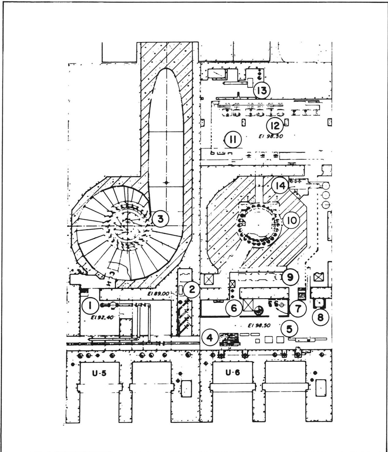
**Fig. 18 Powerhouse Equipment Arrangement**
