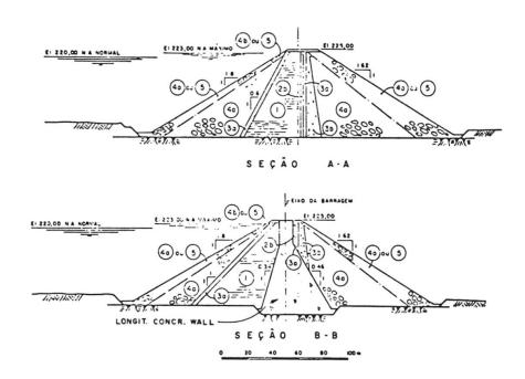
Fig. 10 Cross-sections of overlap between rockfill dam and main (concrete) dam
