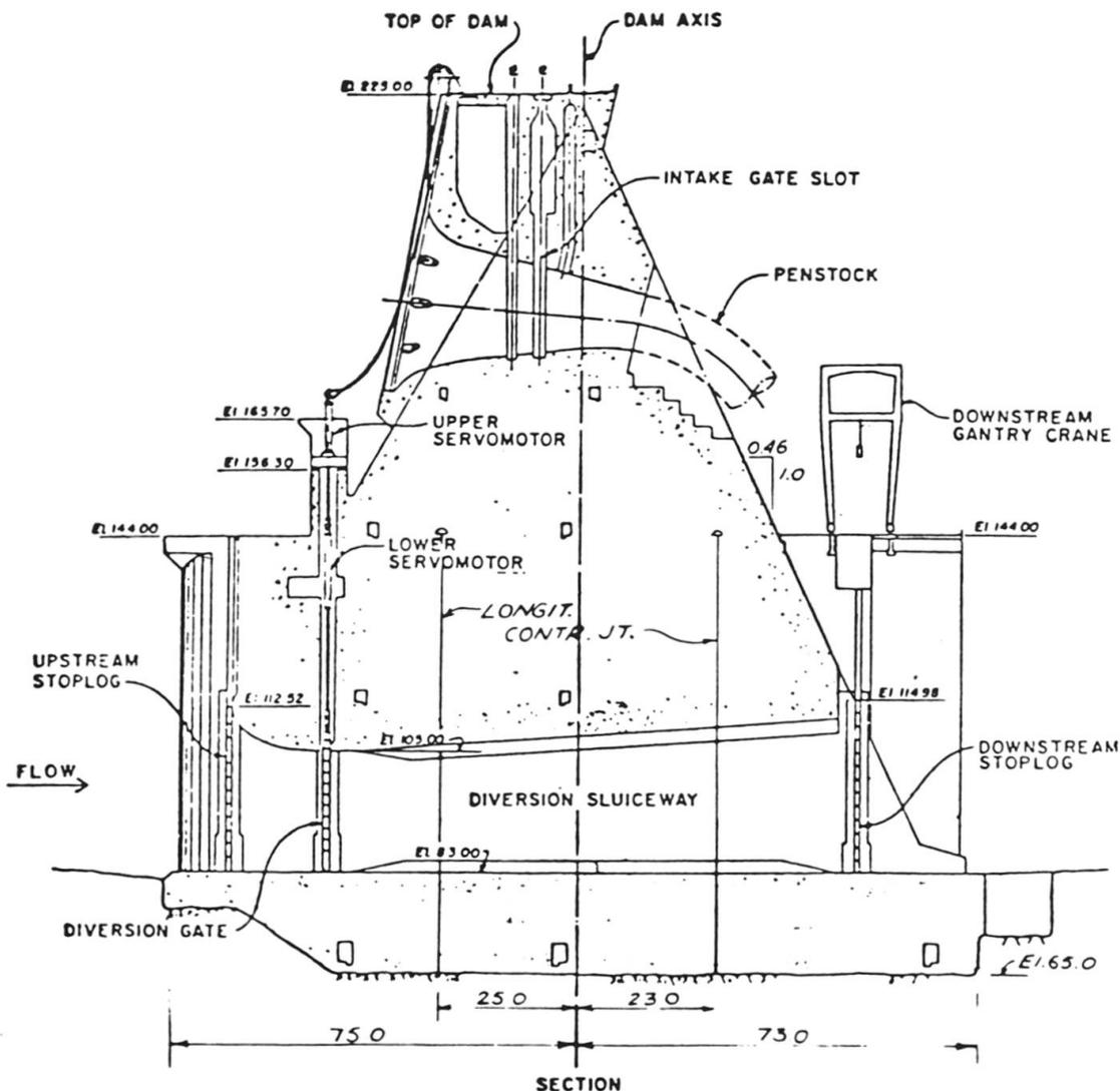
Fig. 7 Diversion control structure
