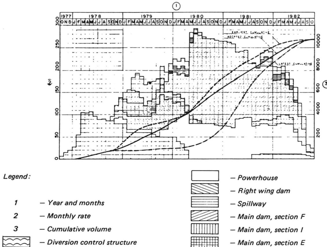
Fig. 4 Adopted Concrete Placement Histogram
