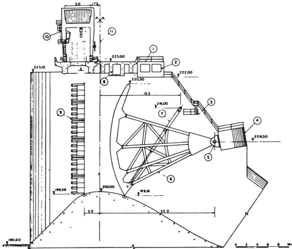
Fig. 3 Spillway Gates
