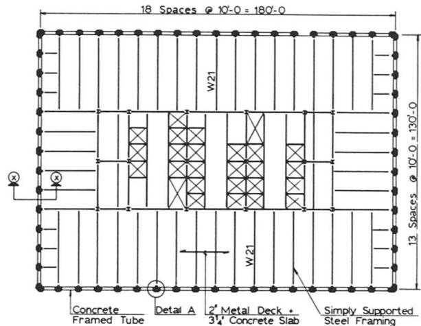
Fig. 2 Typical floor framing plan – One Shell Square building
