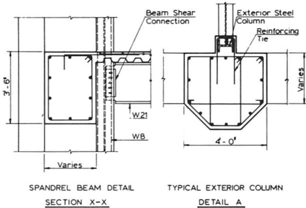
Fig. 3 Exterior beam - column details
